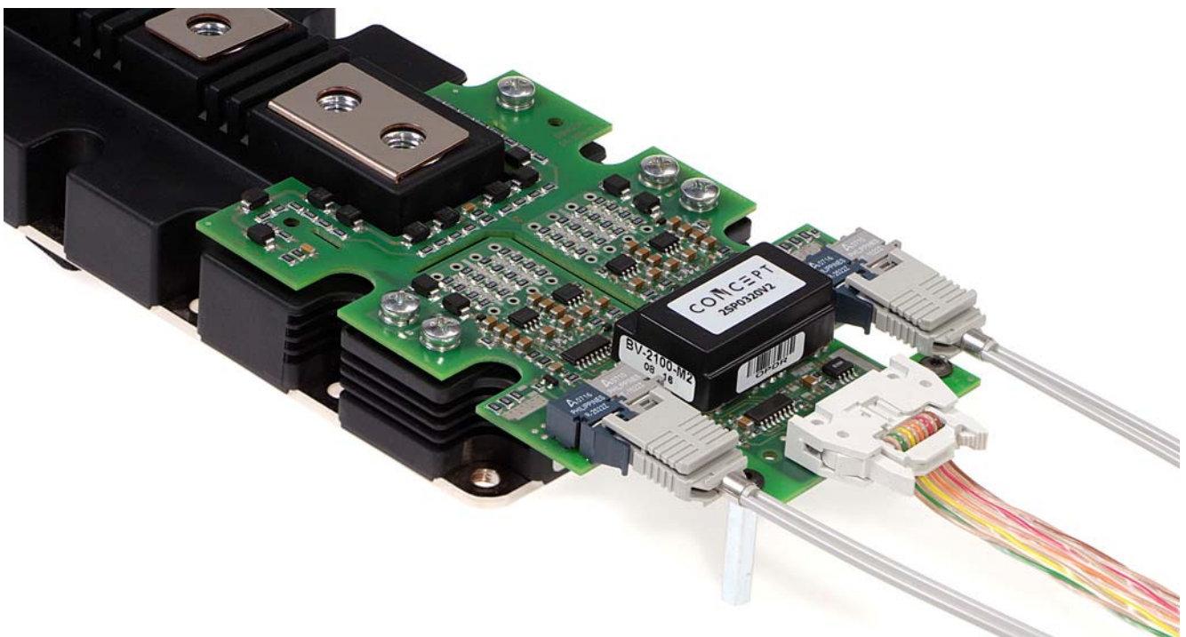
Fig. 13 Additional measures for fixing driver and power-supply cables as well as the relevant version of interlocking fiber-optic links for the 2SP0320V
